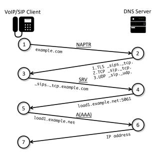
Fig. 1. RFC3263: DNS queries to locate an User-Agent Server
